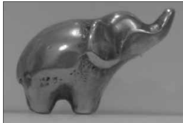
Figure 1. Surface porosity visible on a casting
