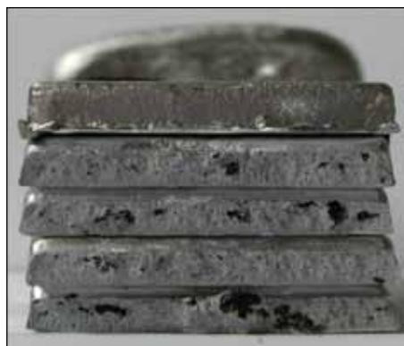
Figure 11. K- Mould sample taken from swarf melted alloy showing the oxide inclusions. Metal Cleanliness Index of this melt was MQI 8
