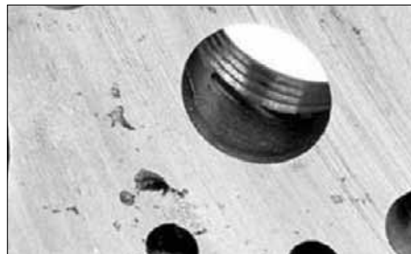
Figure 2. Internal porosity visible on a machined face
