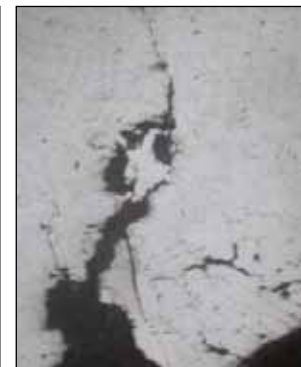
Figure 6. An oxide film travelling deep into the casting wall, potentially resulting in pressure test failure
