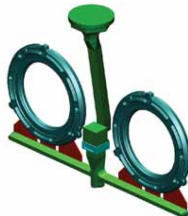
Figure 2 Gating system with cross-over and inclined downsprue
