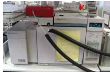
Figure 9b Condensates / tar collected by means of COGAS and determined by GC/MS
