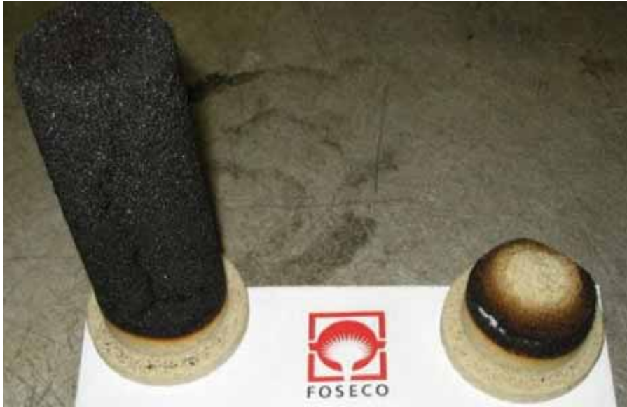
Figure 7 Stage 1 resin bonded core (left) vs. stage 2 resin bonded core (right)
