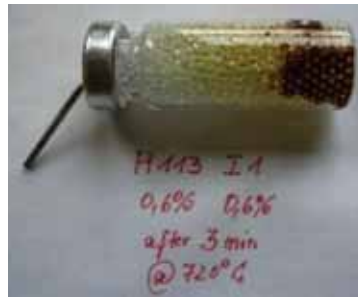
Figure 9a COGAS test: binder residues collected in cooling trap
