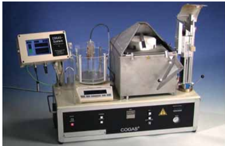
Figure 4 COGAS-device for determination of gas and condensates
