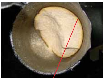
Thin-walled casting and chunky core lead to poor thermal impact on the binder
